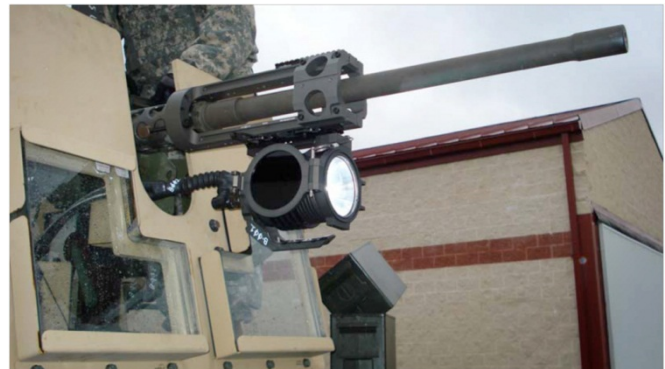
Figure 1. (Upper photo) Handheld searchlight 1 , and (lower photo) searchlight mounted on a vehicle's crew served weapon 2 . ( 1 Photo by APHC Nonionizing Radiation Program) ( 2 Photo by Army Program Executive Office Soldier.
